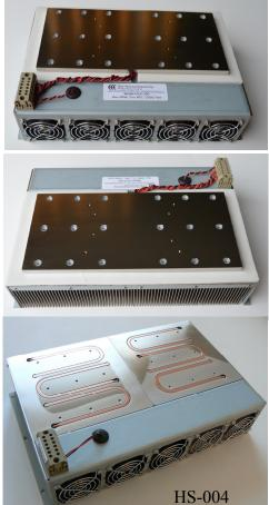
The heatsink we use for OCP-300 is our model HS-004. HS-004 has six heat pipes embedded in the base of the heatsink to minimize heat spreading resistance; the heatsink is nickel plated and the heat pipes are soldered into the heatsink. HS-004 is available for sale as a standalone unit. It is a great solution for high power lasers, electronics, IGBTs, etc.
